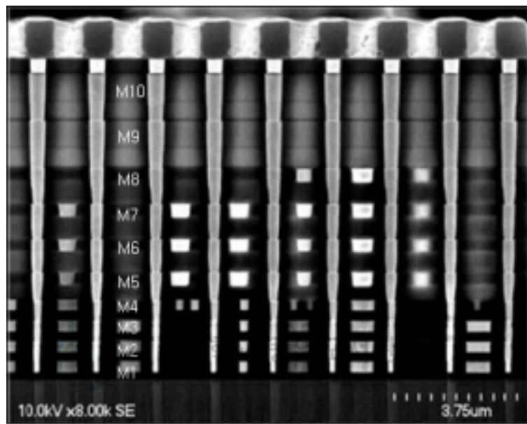
Fig. 1. Cross-sectional SEM picture of 10-level Cu dual-Damascene structure fabricated using SiLK™ at the lower level (minimum feature size from M1 to M4) of multilevel interconnects.
