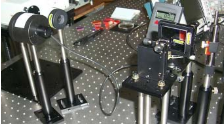
.Fig. 4-28 Emitting power measurement of the solid-state dye laser
