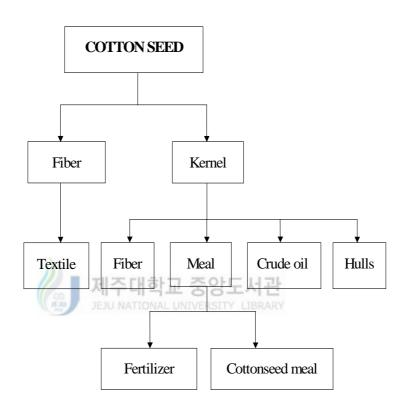
Fig. 2. Processing of cotton and its products
