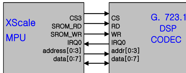
Fig. 21. Connection between MPU and speech codec
