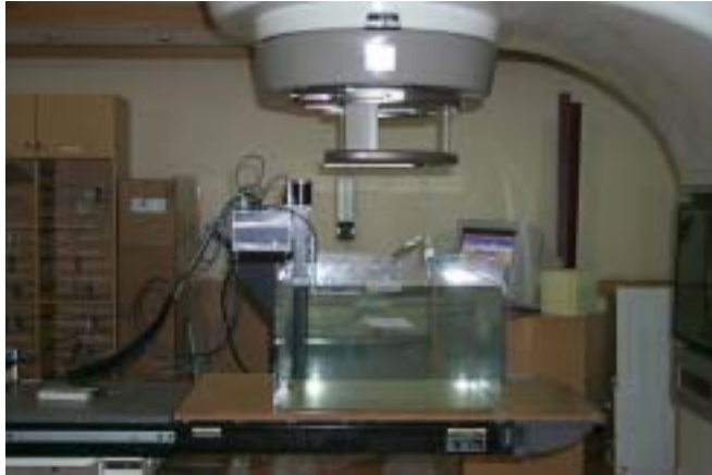
Fig. 6. Water phantom setup for photon measurement.
