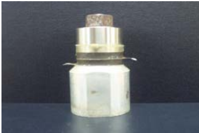
Photo. 3. Photograph of inner bolted langevin transducer
