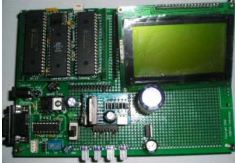
Fig. 3-9 Controller of solar position tracking system
