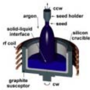
Fig. 2 Growth way of single crystal by using the Czochralski method
