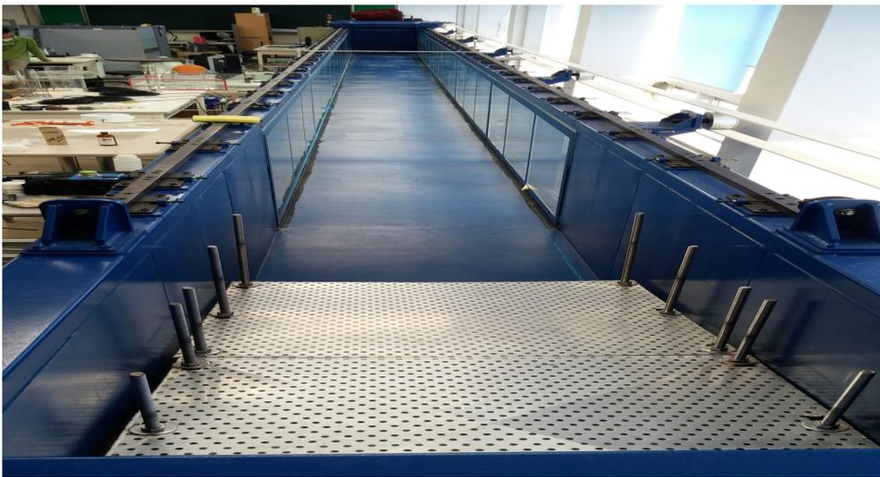
Fig. 7 Beach type wave absorber in 2-D wave tank
