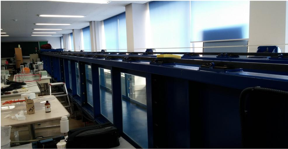
Fig. 5 2-D Wave tank
