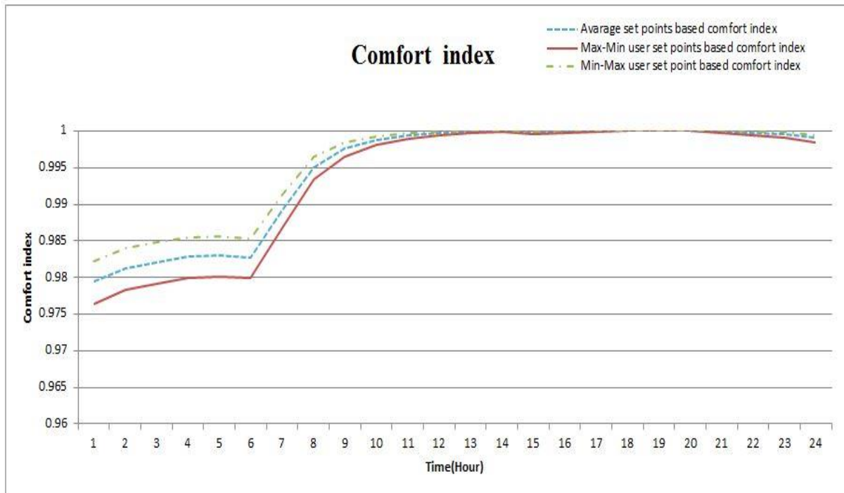
Figure 4.25 Comparison of comfort index of dynamic user set point settings and RBO for multi-users
