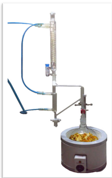
Figure 7. Picture of essential oil determination apparatus.
