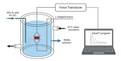
Figure 7. Myography system for measuring the vascular reactivity.
