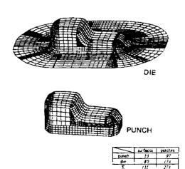
Fig. 2. Schematic view of the parametric tool surfaces for oilpan deep drawing.
